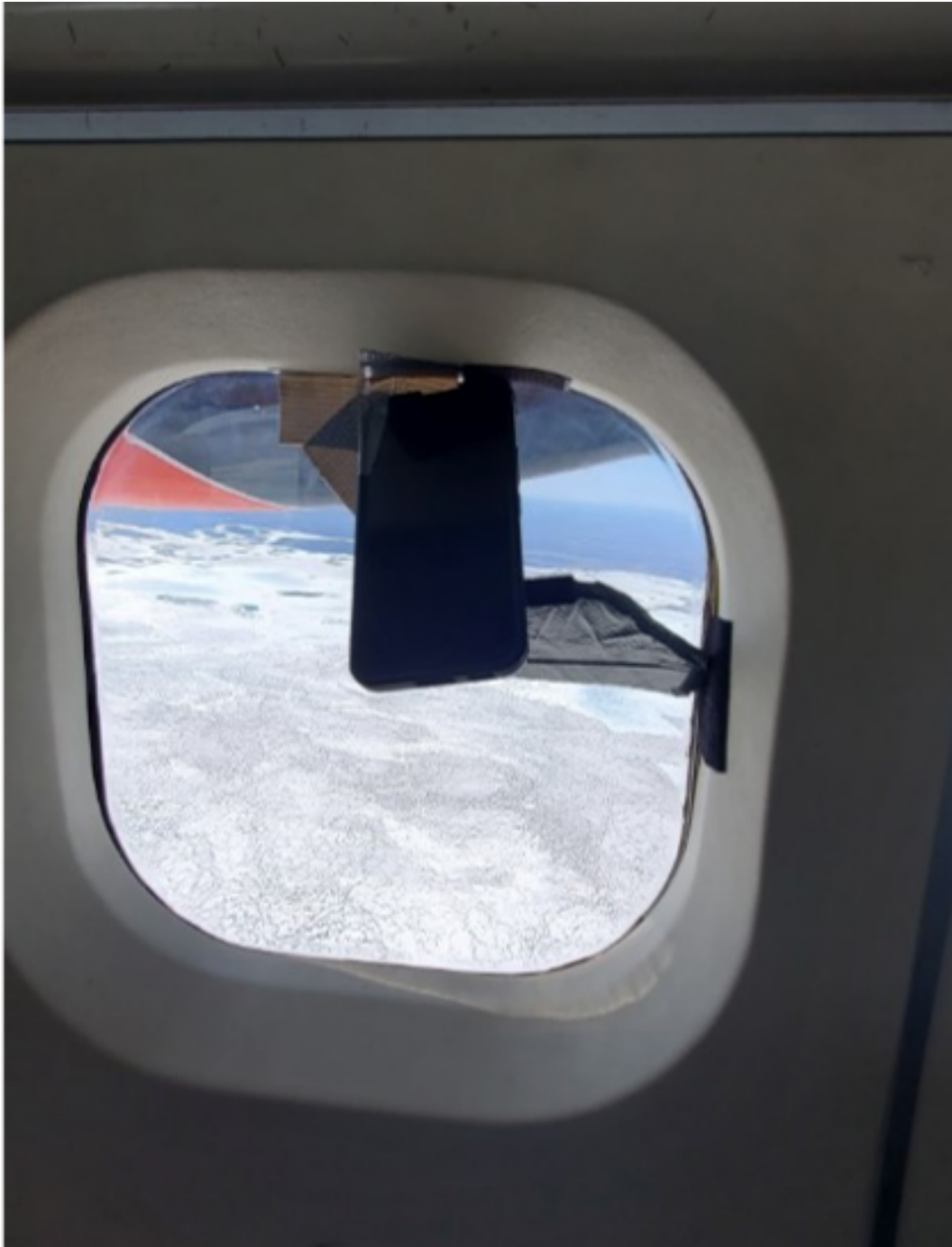
Figure 8. A Samsung S22 smartphone mounted on the window on the right side of the data recorder's seat (Right), and the camera's view of the ground and strut from this same position (left).
