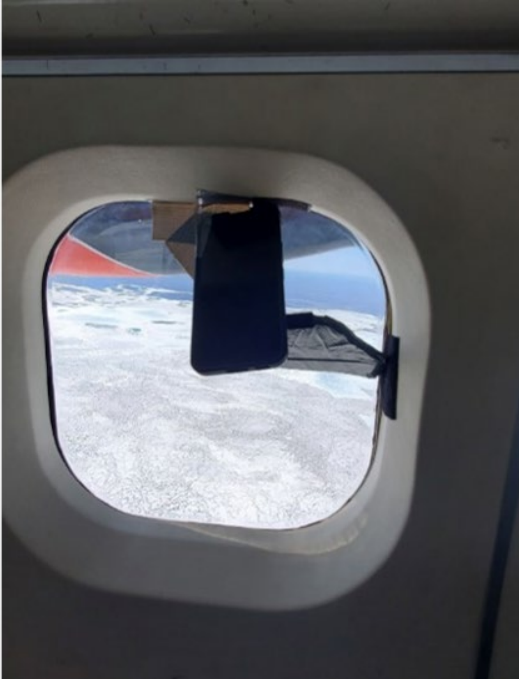
Figure 8. A Samsung S22 smartphone mounted on the window on the right side of the aircraft at the data recorders seat.
